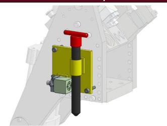
This Pin Package is designed for holstering the lock out pin and securing a "Cube-Style" proximity sensor. The pin is made of high strength steel and certified for usage with TR80 and TR100 pivot applications. The package mounts directly to the pivot using the holes provided. The customer provides the sensor and fasteners.
