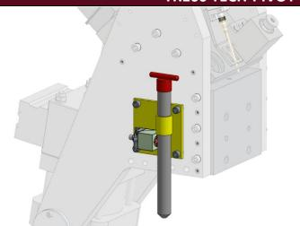
This Pin Package is designed for holstering the lock out pin and securing a "Cube-Style" proximity sensor. The pin is made of high strength steel and certified for usage with TR160 applications. The package mounts directly to the pivot using the holes provided. The customer provides the sensor and fasteners.
