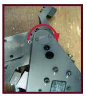
Rotate arm assembly clock-wise to get access hole to third bolt.
