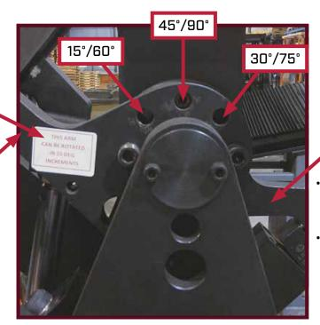
This arm (ADL005) is **stationary** as shown in the chart. **The arm is marked on the outside face for arm positions.**
