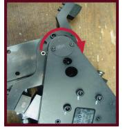
Rotate arm assembly clock-wise to get access hole to third bolt.
