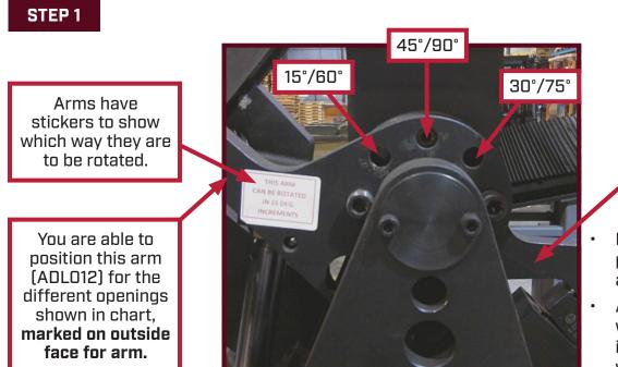
This arm (ADL005) is stationary as shown in the chart. The arm is marked on the outside face for arm positions.
