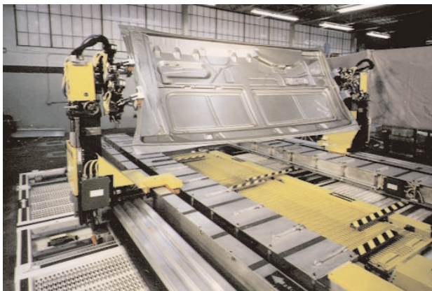
Flexcart 4.1 with Gripper Heads securing part.
